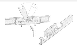
Turning the fork wrench clockwise will press the roller to be adjusted against the top raceway which will set the roller carriage free of play. Excessive pre-tensioning must be avoided because this will increase friction and reduce the useful service life. 10. Before reinserting the roller carriage, make sure that the raceways / rollers are properly lubricated using a heavy duty lubricant for linear guidance.
